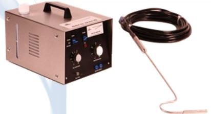
**VC - Aero 5000 and 1300** - These generators produced an aerosol to EN-ISO 14644-3 for filter testing applications, They are available in a number of configurations, at outputs to suit small to large scale air flows. The particle size remains extremely consistent across the entire range.
