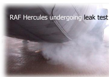
RAF Hercules undergoing leak test
