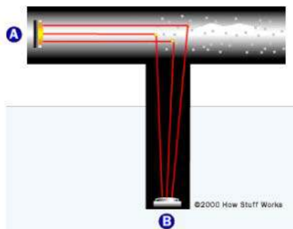
Figure 3 - Photoelectric Smoke Detector Schematic [12]
