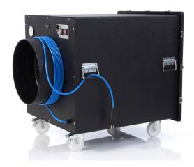
For many years Concept have produced specialist aerosol and smoke generating equipment for the chemical, biological and nuclear industries, for testing the efficacy of the HEPA filters in these cleanroom environments.
